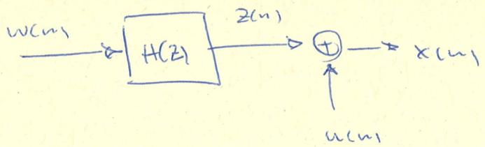
$$Y_x(n) = Y_2(n) + Y_{w(n)} = \Gamma_w^2 S(n) + \frac{4}{5} Y_2(n-1) + \Gamma_u^2 S(n)$$
