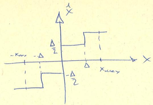
$$\sigma_{gx}^2 = 2 \int_0^{\Delta} \left( x - \frac{\Delta}{2} \right)^2 f_x(x) dx + 2 \int_{\Delta}^{x_{max}} \left( x - \frac{3\Delta}{2} \right)^2 f_x(x) dx$$
